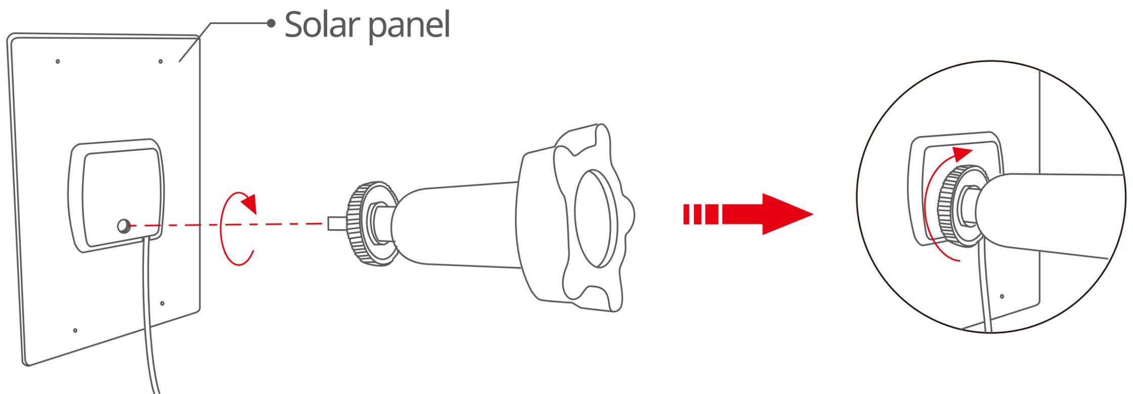
4. Rotate the locking screw cap into the base. Make sure that the universal joint is angled upward.
