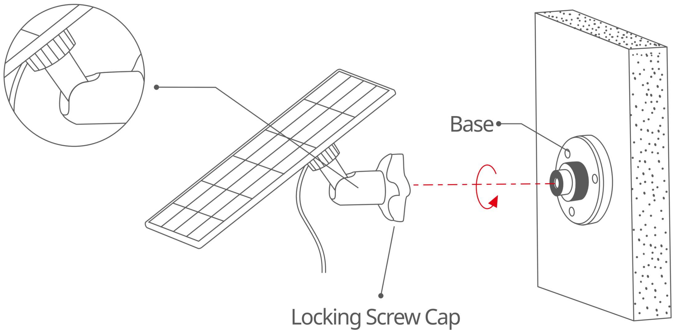
5. If you want to adjust the position of the solar panel, loosen the locking screw cap first, then rotate the sleeve rod, and tighten the locking screws cap when the panel is in position.
