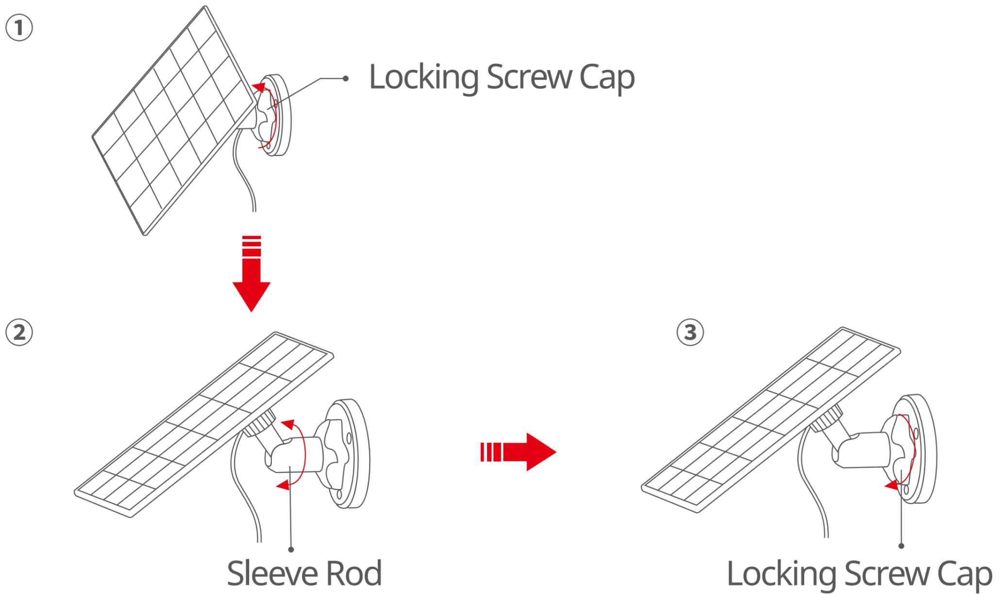
6. When completed, please check that all the locking mechanisms are tightly secured.
